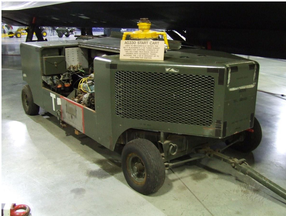
Image 4: An AG330 Start Cart with 2 Buick nailhead engines inside. Later A-12 derivatives used the same or similar start cart. (Source: Jaydec at English Wikipedia)
